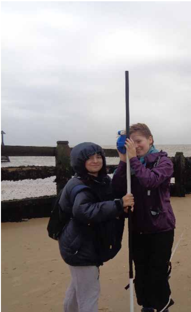
Beach gradient measurements along a transect line in gale force winds.
