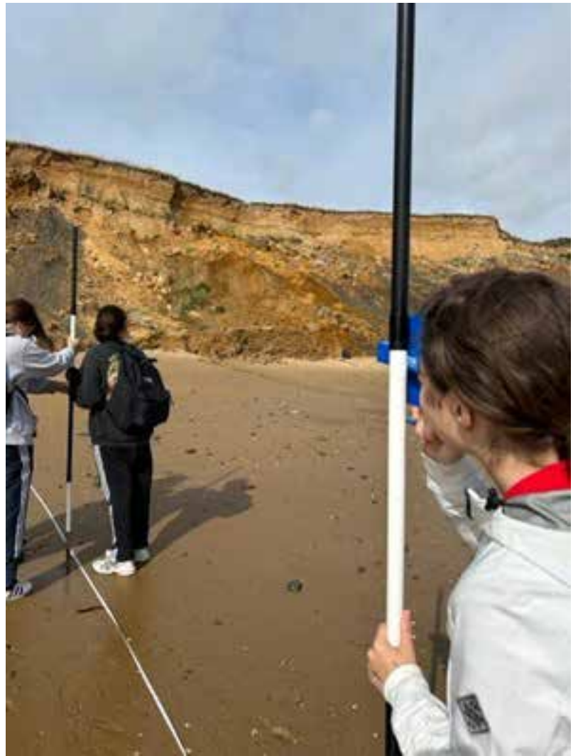
Beach gradient measurements along a transect line in gale force winds.
